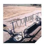
Wire rope style railcar positioner Alternately, a wire rope cable and drum arrangement is used to move the positioner.
