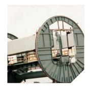
Integral platen weigh scale Integral load cells allow railcars to be weighed before and after dumping without the need of separate track scale. Excellent accuracy of 0.1% meets strict railroad requirements. Platen does not interfere with dumping operation.
